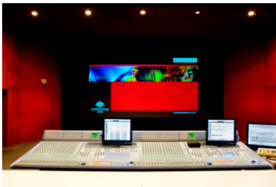
ICON dual operator 32-fader D-Control in AFTRS mix theatre
